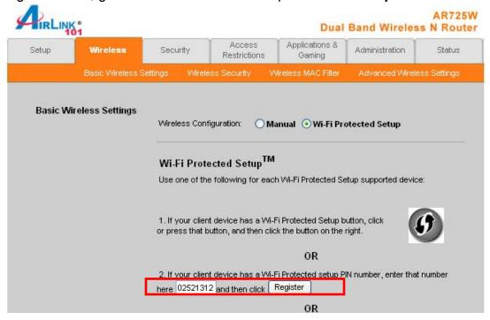
The router will start to search for the WPS enabled device with matching PIN code.
